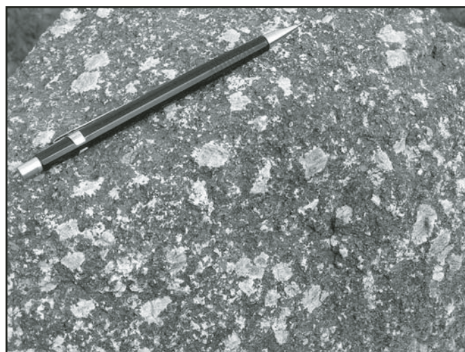
Figure 44. Isotropic-textured troctolite containing large crystals of anorthitic plagioclase, southern part of the Green Acres gabbro, central Perris block.
