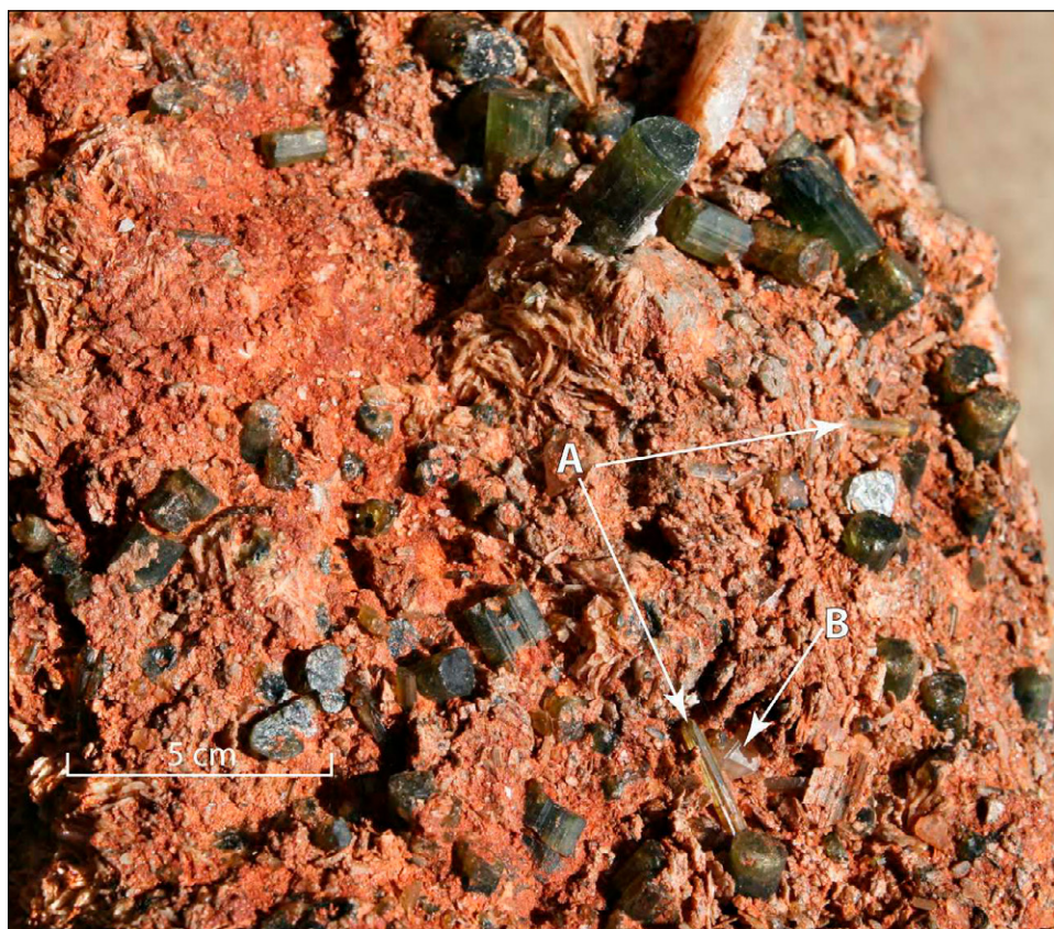
Figure 28. Cavity wall segment from cavity in upper part of a chimney, showing first-generation elbaite (larger, dark-green crystals), second-generation elbaite (A arrows), and second-generation quartz (B arrow). Orange material is hypogene montmorillonitic clay.
