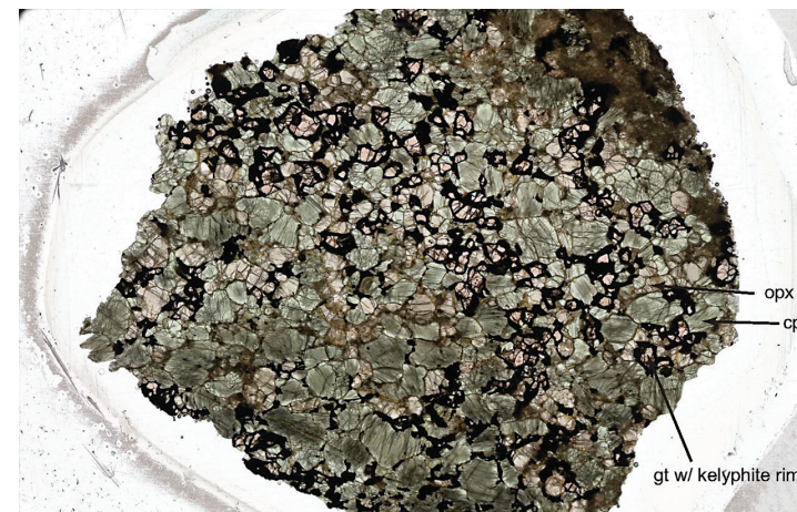
Figure S-2 Plane-polarised light photograph of thick section (~200 \mu\text{m} ) of high-MgO websterite BC98-5.
